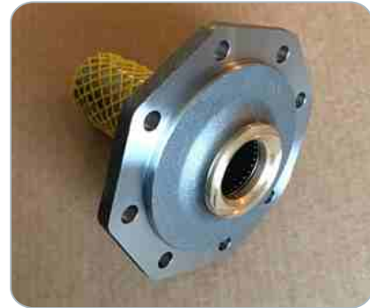
FRONT SPINDLE LANDCRUISER 43401-60080/40 WITH BUSH
