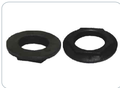
Axle Nut trailer (1=LH; 2=RH) Size : 60x2 p
