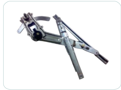
EOMC-15 MITSUBISHI CANTER Glass Model- 4D31 Regulator R/H Part No.- MB394571
