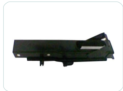
EOMC-45 MITSUBISHI CANTER Bracket, Clutch Model- 4D31 Pedal Upper Part No.- MB334596
