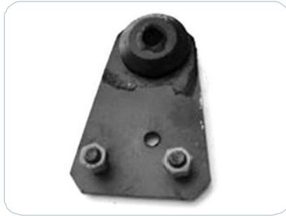
EOMC-26 MITSUBISHI CANTER Cushion Radiator Model- 4D31 Part No.- MB390080
