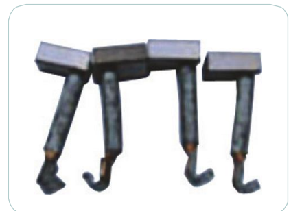
EOMC-326 MITSUBISHI CENTER Starter Brush Set Model- 4D32 Part No.- ME701576
