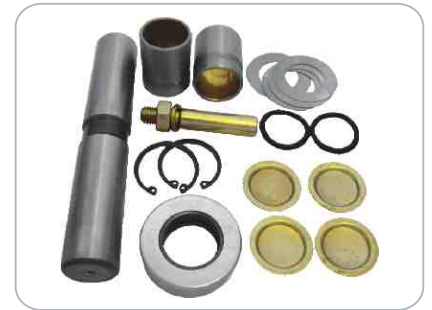
KING PIN KIT EOKPK-30 OM 364 PIN SIZE - 30 x 171.2 mm
