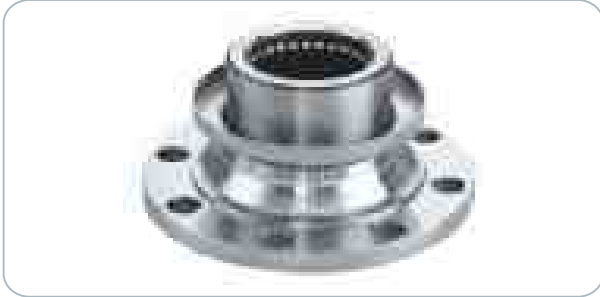
DIFFERENTIAL AXLE FLANGE 8 BOLT - M16 O.E.M. PART No. 355 350 06 45 Ø 165mm 81.39115-5025 Z - 28 EOCP-062 DIN 5482 60x55
