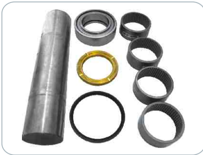
KING PIN KIT EOKPK-31 O.E.M. PART No. 6553300519 / S1 ACTROS (ROLLER BEARING) PIN SIZE - 50 x 223 mm
