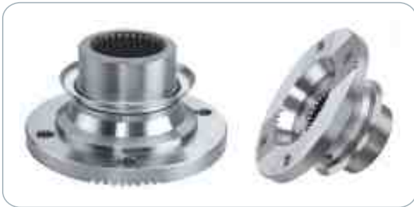
DIFFERENTIAL AXLE FLANGE O.E.M. PART No. 355 353 2445 EOCP-074 4 BOLT Z - 26, Ø 165mm DIN 5480 55x51 STAGGERED TEETH
