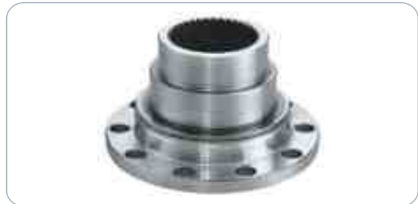
GEAR BOX ZF OUTPUT FLANGE 10 BOLT - M16 O.E.M. PART No. 1295 338 059 Z - 36, Ø 180mm 000 264 37 45, 81.39115-0214 DIN 5480 71x75 EOCP-059
