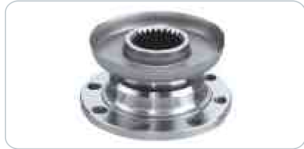
CENTRE FLANGE O.E.M. PART No. 336 410 00 30 EOCP-071 8 BOLT - M12 Ø 150mm Z - 26 DIN 5482 55x50
