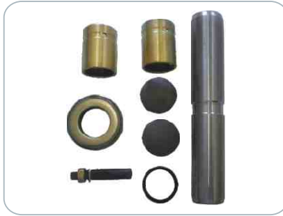
KING PIN KIT EOKPK-57 O.E.M. PART No. 316 330 0119 PIN SIZE - 30 x 186.5 mm
