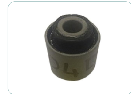
EOBH310 HONDA OEM No.: 31126757551 BUSH REAR TRAIL ARM HON BALL CIV UPP
