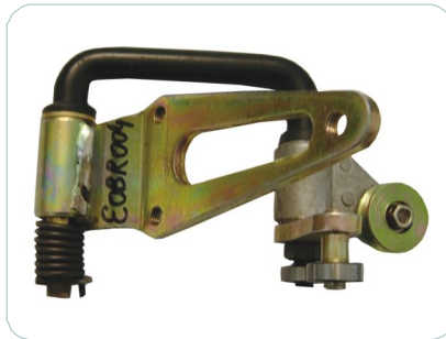
NISSAN SLD. DOOR BRAKET, NISSAN E-20, AUT TYPE EO. Part No.: EODB014
