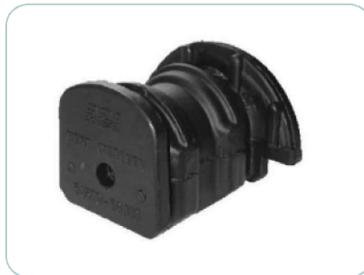
EOBH59 NISSAN Lower Control Arm Bush - Front Outer OEM No.: 54560-50A00 SENTRA
