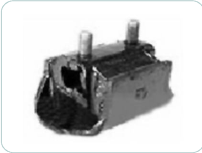
EOMTG162 Transmission Mounting FORD OEM No.: UH71-39-340 COURIER, RANGER, MAZDA, 323, B1600, B1800, B2000, B2200, DRIFTER
